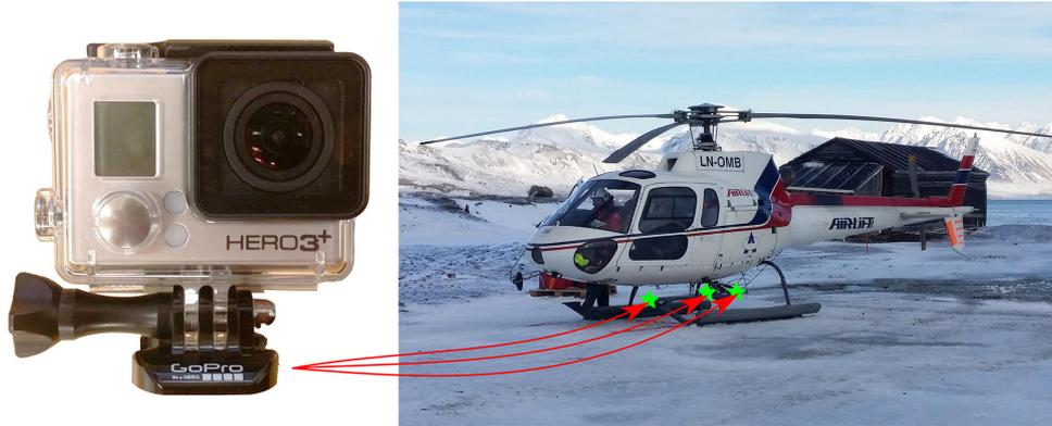
Figure 31: GoPros attached to a helicopter
