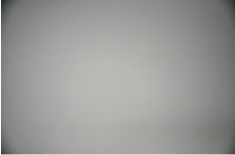
Figure 7: Vignetting effect on an homogeneously gray, evenly lit surface (Nikon D90 with Nikkor 18-105 VR at 18mm-f/3.5)
