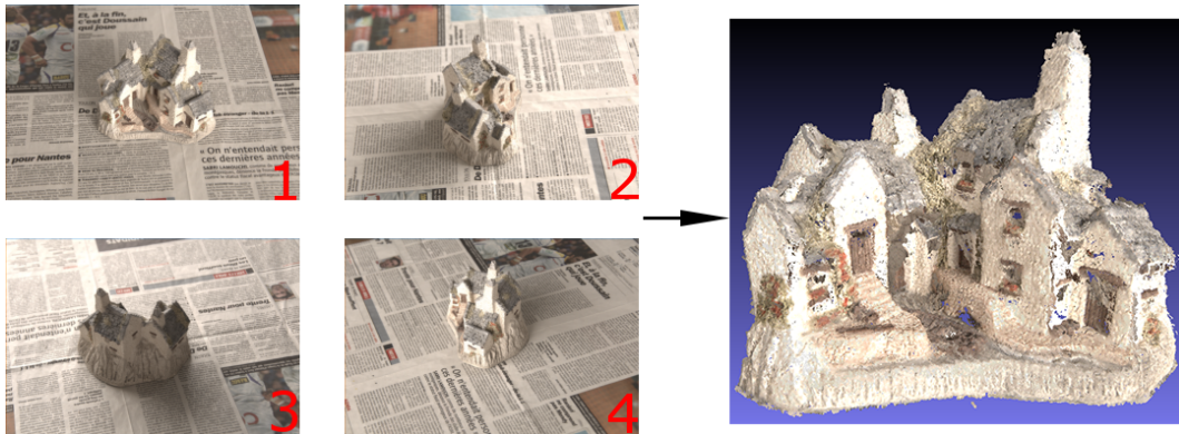
Figure 24: Sample images for the computation of a 3D model of a miniature house and resulting model - from [Girod and Pierrot-Deseilligny, 2014].
