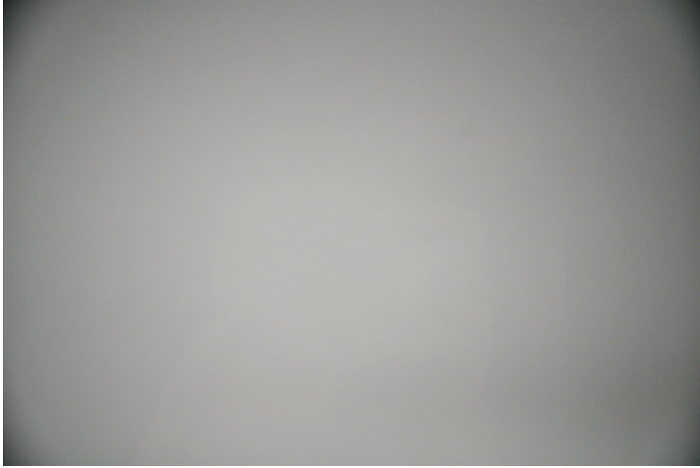
Figure 12: Vignetting effect on an homogeneously gray, evenly lit surface (Nikon D90 with Nikkor 18-105 VR at 18mm-f/3.5)
