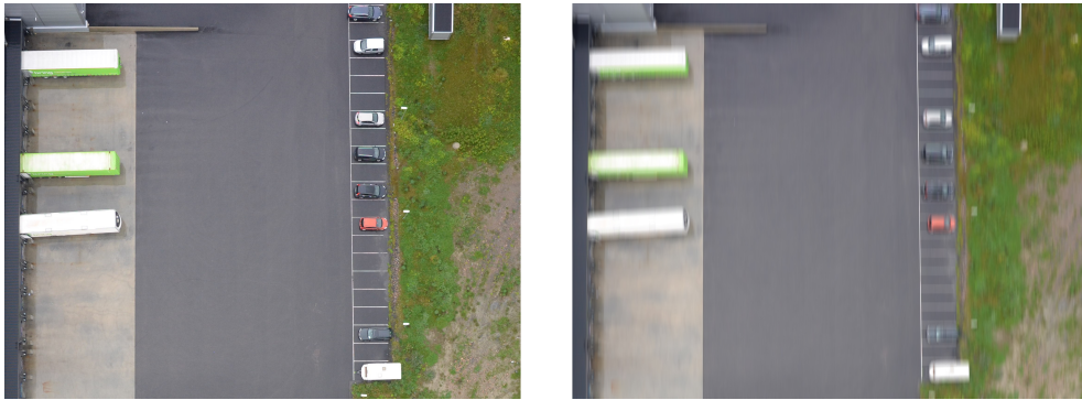
Figure 34: Example of a 4 pixel motion blur
